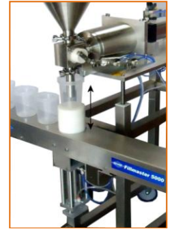
Container lift mechanism
