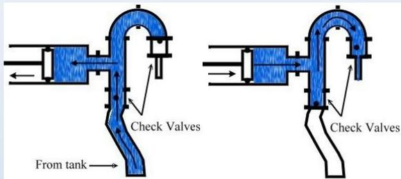
Each fill cycle starts as follows. The piston (inside the fill cylinder) takes an intake stroke. It draws product through the intake tubing, opening the lower check valve and closing the upper check valve. Then the piston moves the product from the cylinder by opening the upper check valve and closing the lower one. Piston filling is simple, time proven and very accurate.
